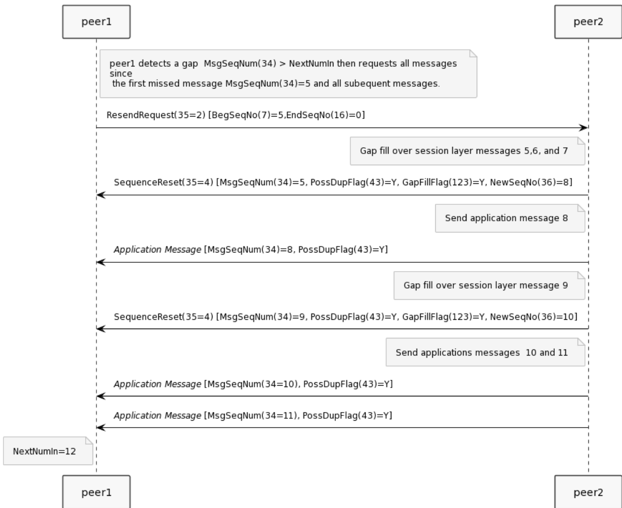
Figure 15 — Example using the SequenceReset(35=4) to gap fill over multiple messages.
