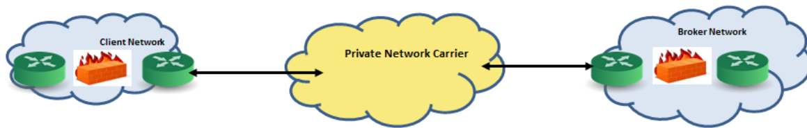
Single Client Point to Point Connectivity via Leased Line Arrangement Through a Private Network
